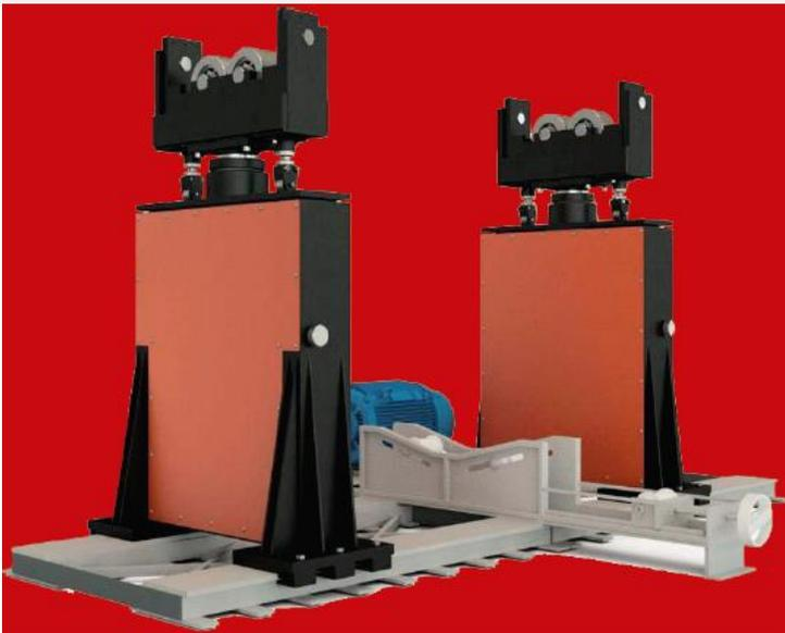
**EI-25T** Balancing Machine can balance all kinds of rotors up to 25 tons.
