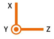
Once that you've placed the sensor on your machine, set it up on Digivibe and define each axis to an orientation: Horizontal, Vertical and Axial.
