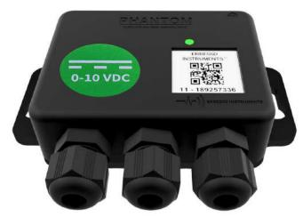
With the General Purpose Phantom you can adapt the data collection to your specific needs. Take **any 0-10V sensor** and make it wireless.
