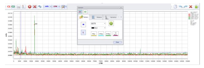
Locate Markers: Allows user to identify Max, Max 3, Max 5 and Max 10 Peaks within an FFT
