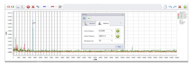
Band Filters: Allows user to apply low pass, band pass, high pass, and band reject filter methods
