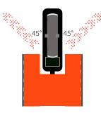
The **SBS** base has the capability to rotate itself within it's axis and has an **horizontal 45° tilt**. These features protect the poles and provide maximum **durability**.
