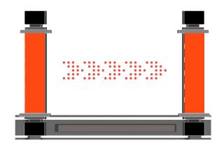
The El 300 pedestals can be adjusted to adapt to a wide variety of shafts.
