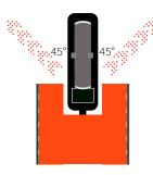
The **SBS** base has the capability to rotate itself within it's axis and has an **horizontal 45° tilt**. These features protect the poles and provide maximum **durability**.
