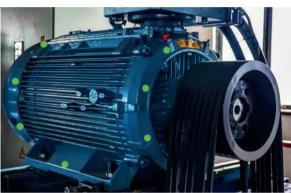
With the help of any accelerometer, instead of a video recording, you can detect **up to 15,000 Hz** in any axis with very high precision. With this, you will be able to detect bearing issues, gearbox problems and many, many more.
