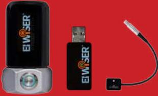
Wireless accelerometer: 2.4 GHz
