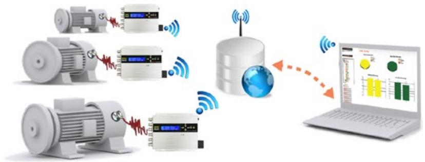
Instruments has created a specific website called EI Analytic that allows the user to remotely access this data and thus determine the condition of the machinery in real time from anywhere in the World.
